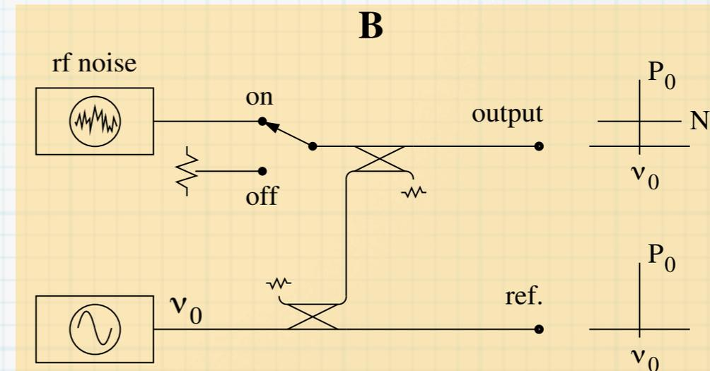
The problem is that the phase detector (saturated-mixer) is sensitive to AM
