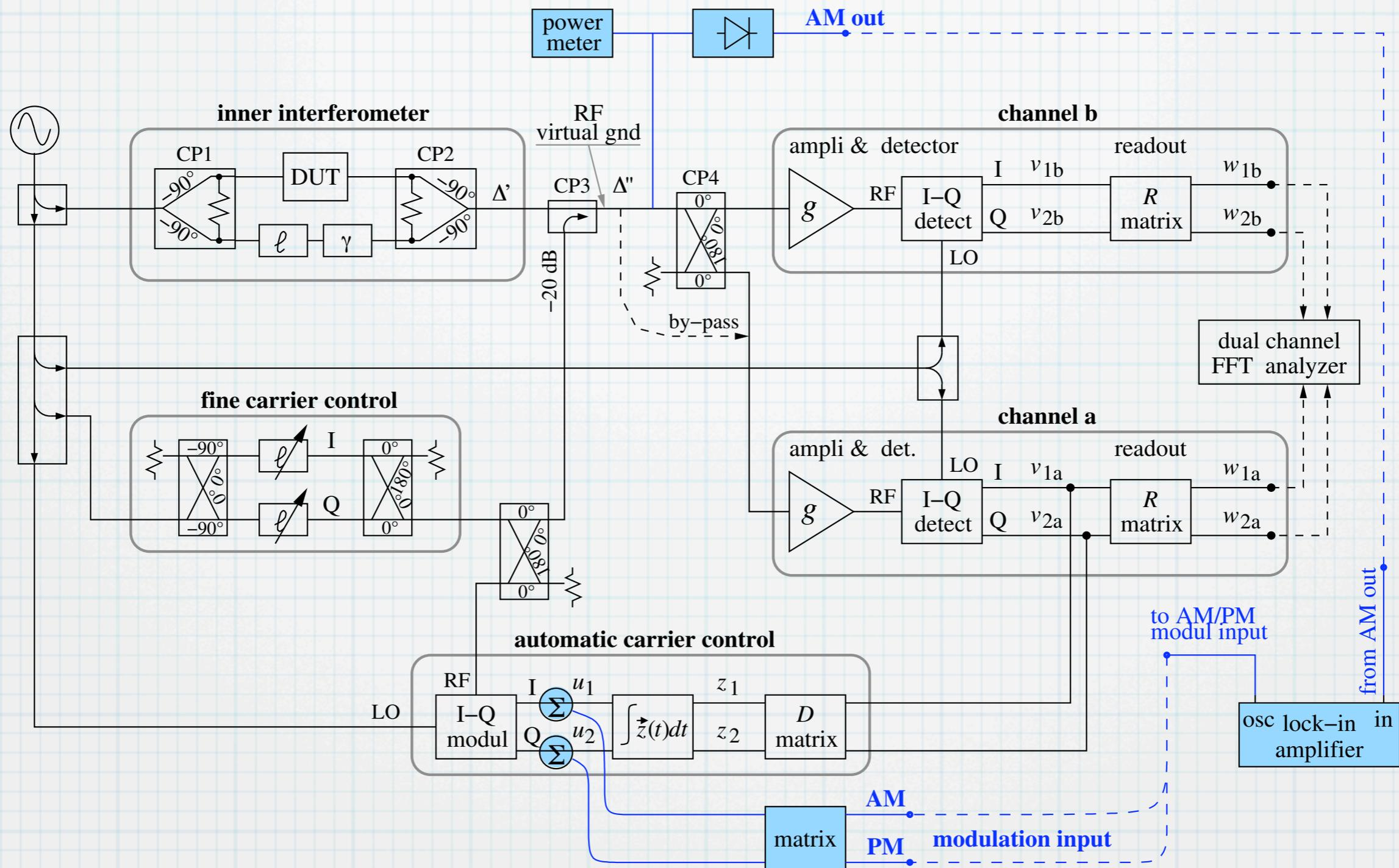
The dual-bridge contains almost all the blocks needed to calibrate the measurement
