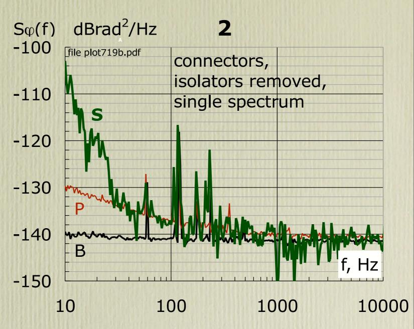
S: example of single spectrum, with optical connectors and no isolators
