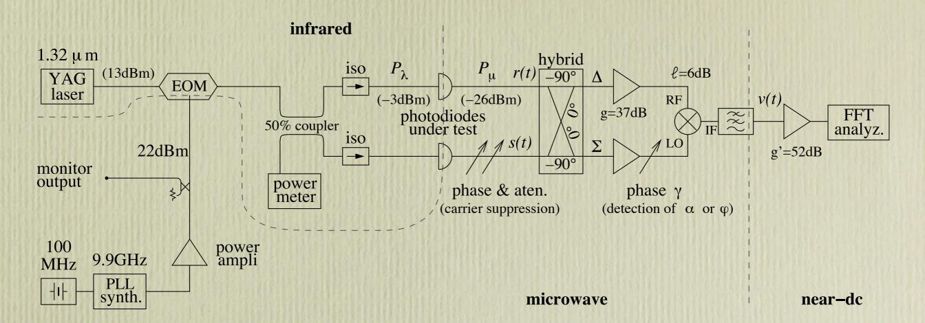
bridge (interferometric) scheme
