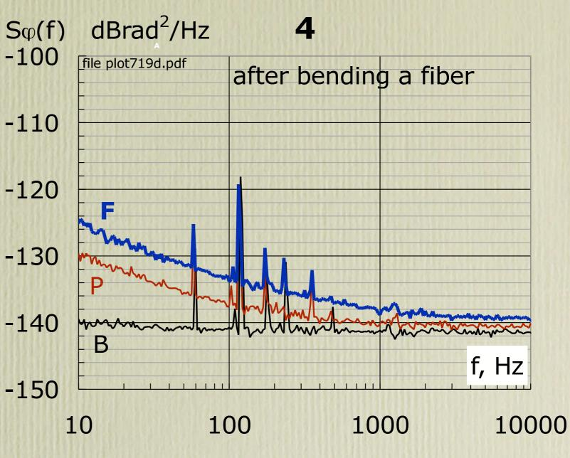
F: after bending a fiber, 1/f noise can increase unpredictably
