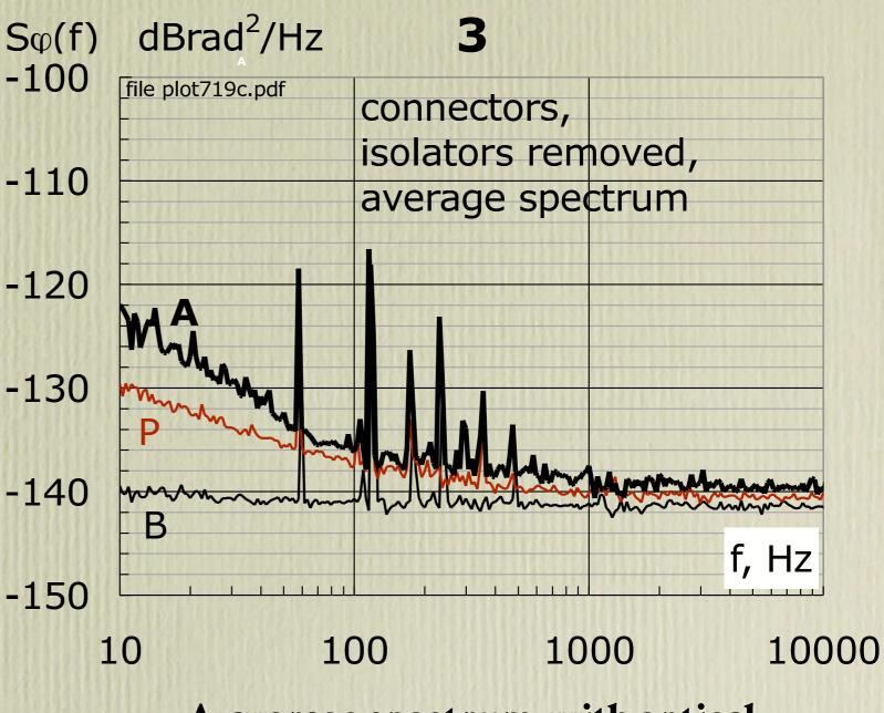
A:average spectrum, with optical connectors and no isolators
