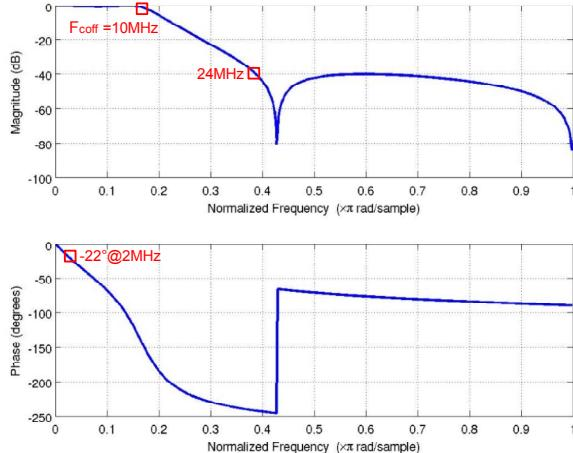
Fig. 4. Low pass filter design specifications. Cut off frequency: 10MHz, stop band attenuation: 40dB. Phase shift added at the desired frequency: 22°.
