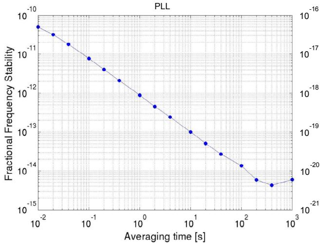
Fig. 7. Allan deviation of the PLL phase noise. Expected frequency stability of the completed system implementation.
