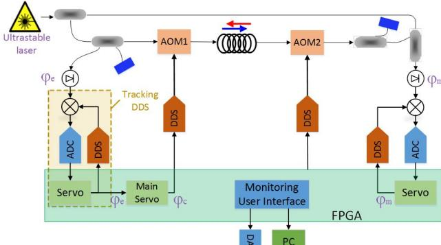
Fig. 1. Doppler compensation implemented by using tracking DDS.
