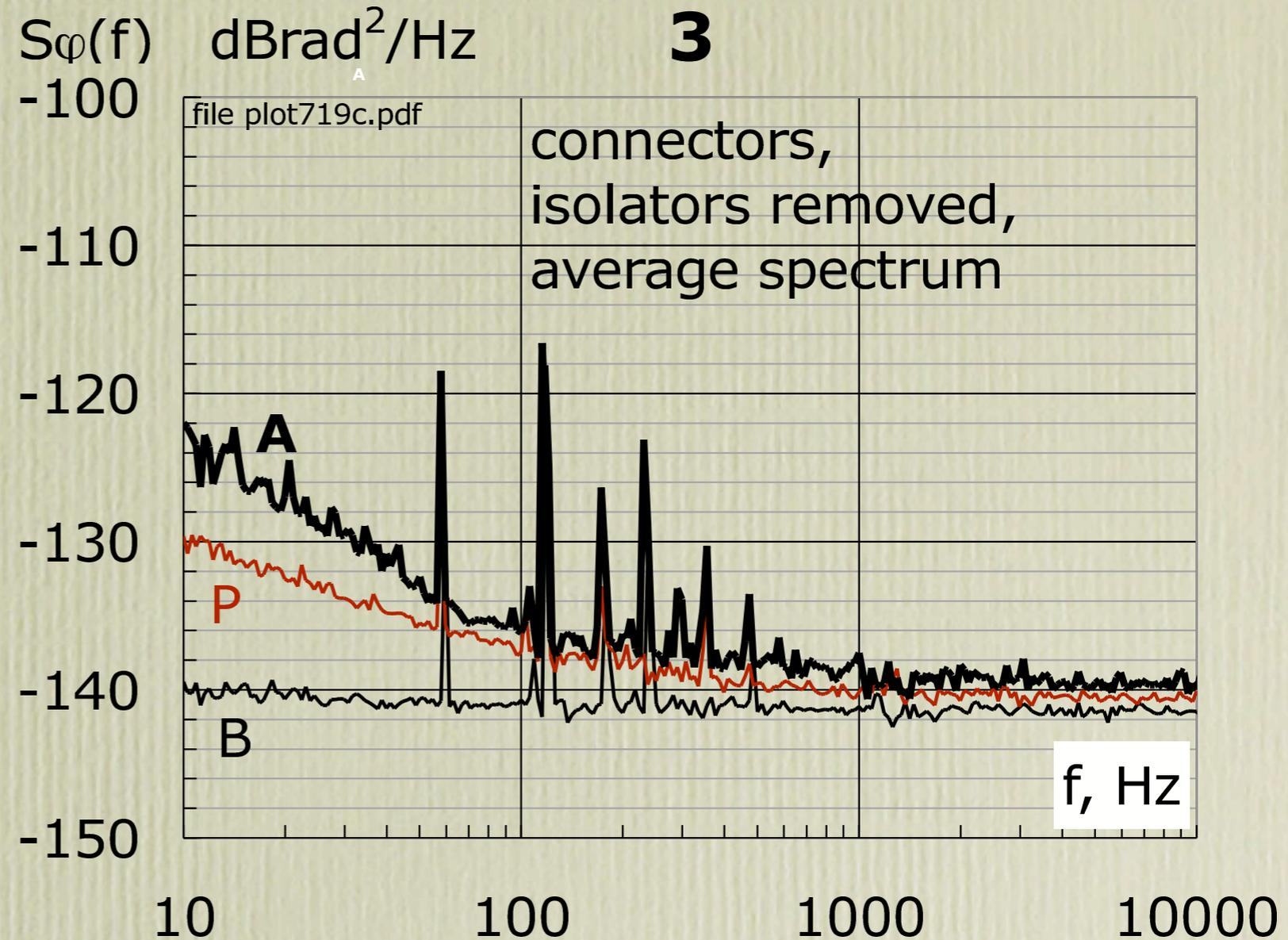
**A: average spectrum, with optical connectors and no isolators**
