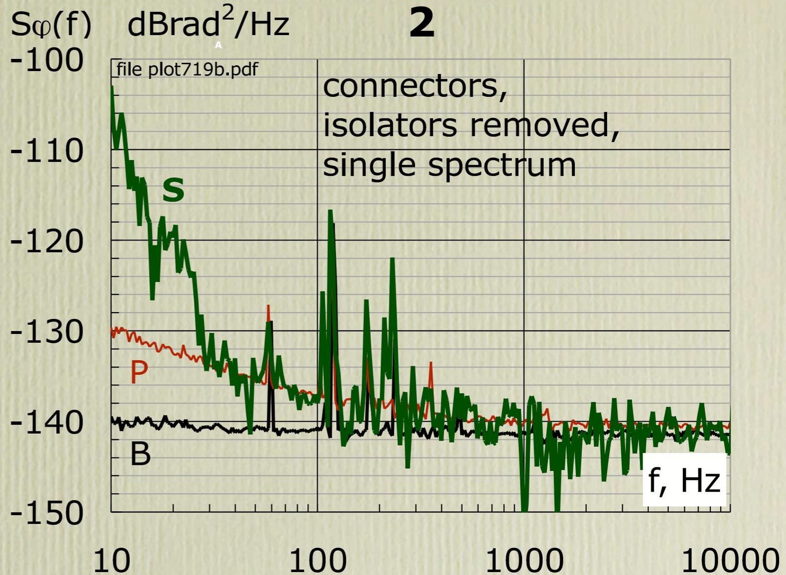
**S: example of single spectrum, with optical connectors and no isolators**
