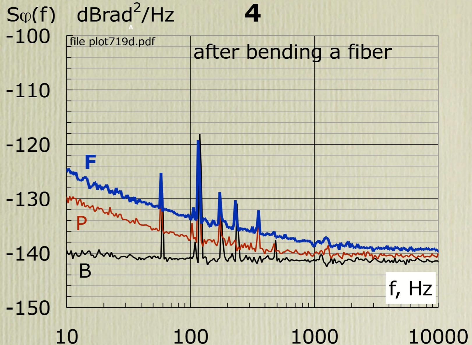
**F: after bending a fiber,  $1/f$  noise can increase unpredictably**
