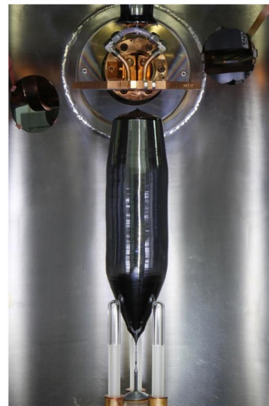
Figure 1. The new float-zone ^{28}\text{Si} crystal Si28-23Pr11 and its cutting scheme. The isotopic enrichment is about 0.999985. To determine density, two spheres (Si28kg01a and Si28kg01b) were manufactured from parts P and S. From the parts L, N, Q, U, and V small samples were prepared for the determination of other crystal properties. The parts U and V contain some cracks (thin irregular lines). No cracks were detected in the parts K to T.
