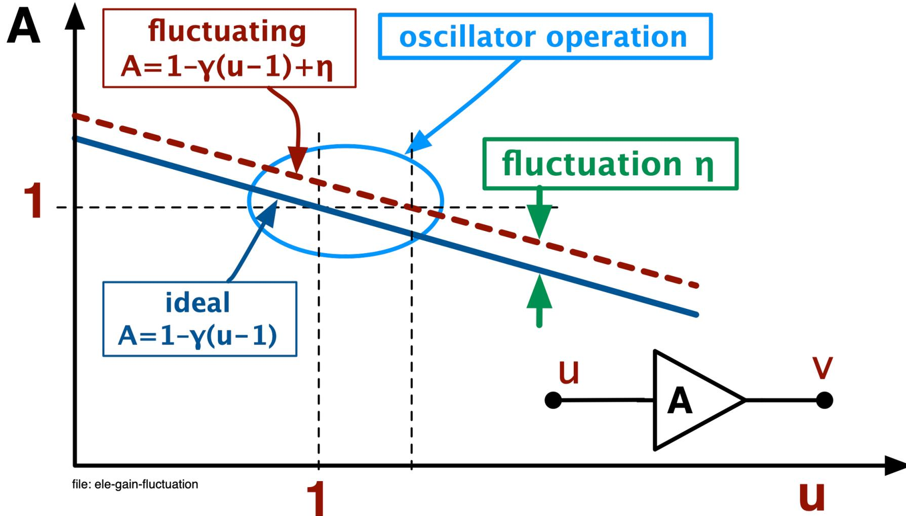
Gain compression is necessary for the oscillation amplitude to be stable
