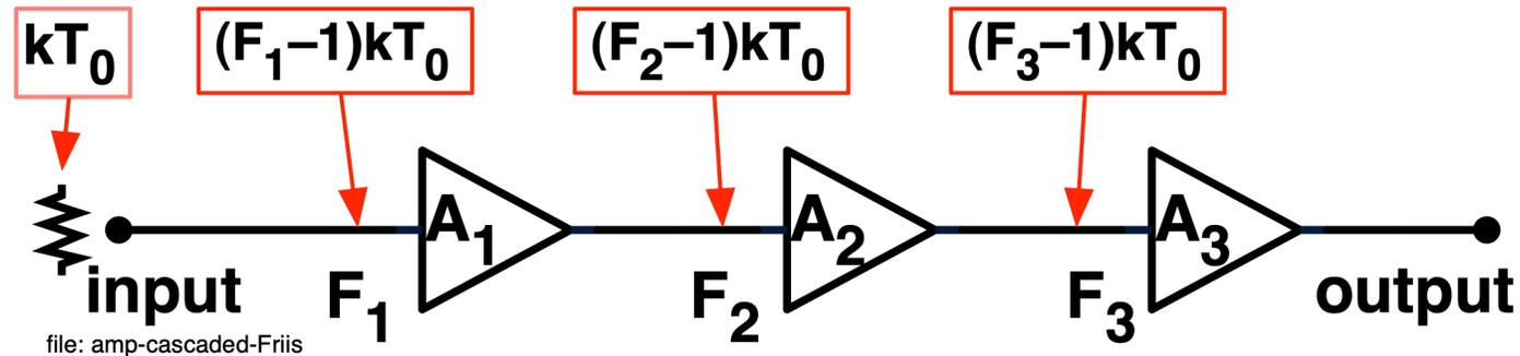
$$N_e = F_1 kT_0 + \frac{(F_2 - 1)kT_0}{A_1^2} + \frac{(F_3 - 1)kT_0}{A_2^2 A_1^2} + \dots$$
