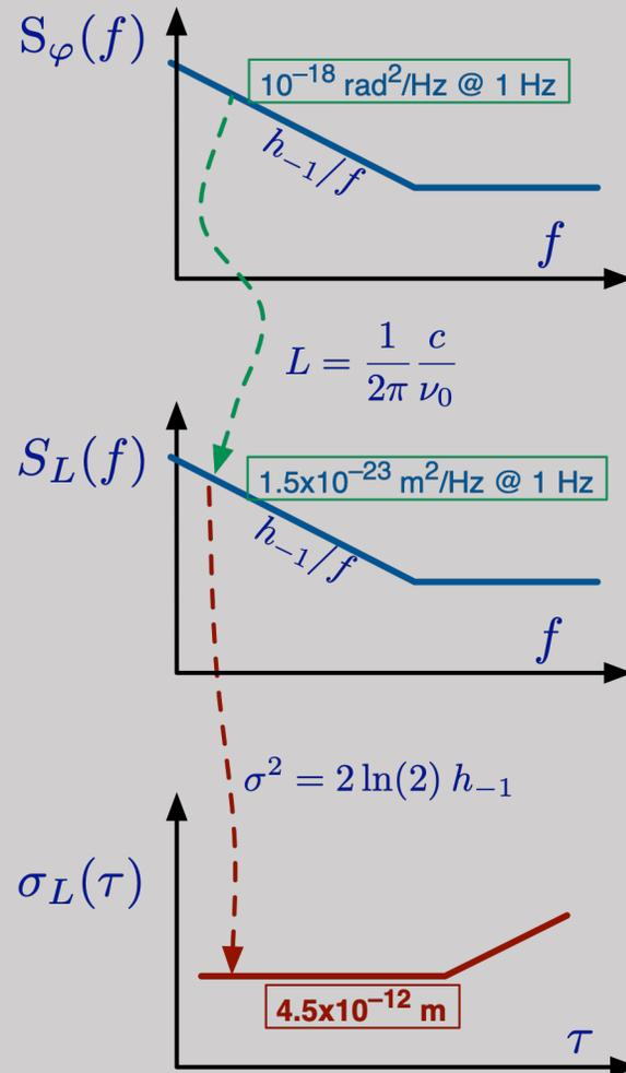
Any phase fluctuation can be converted into **length fluctuation**
