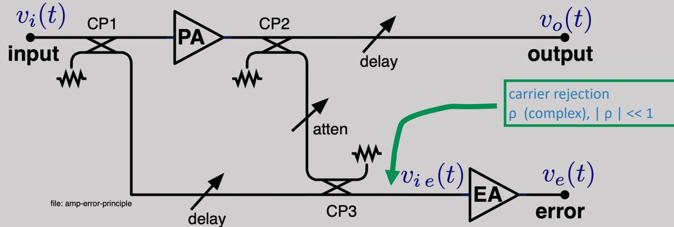
$$(v_{ie})_{PA} = \frac{1}{2} V_i \left\{ a_1 + a_2 [n'(t) + in''(t)] \right\}_{PA} e^{i\omega_0 t} \left( \frac{1}{a_1} \right)_{PA} \quad \text{PA contrib}$$
