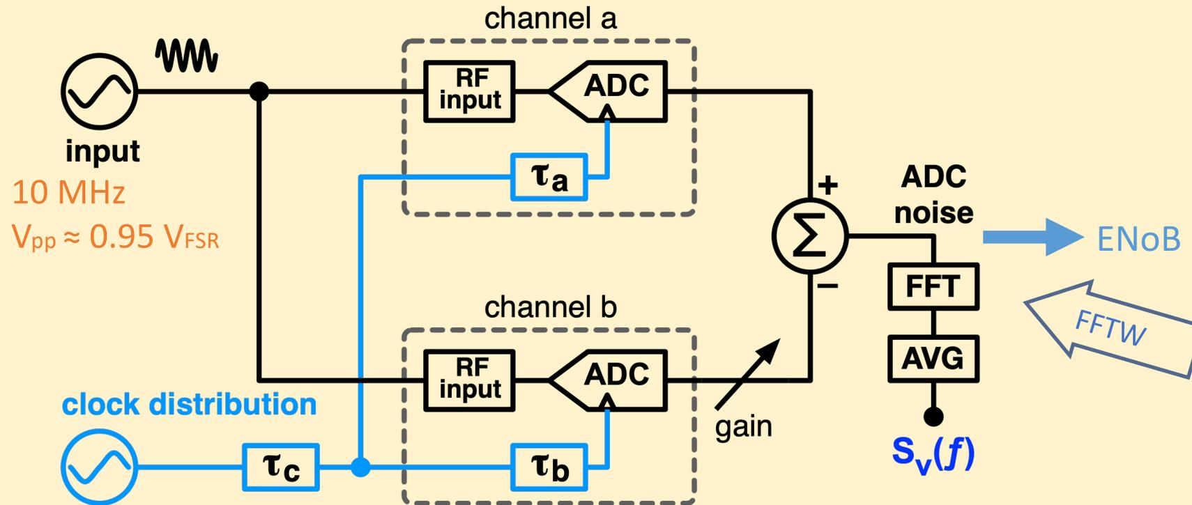
The differential clock jitter introduces additional noise due to the asymmetry between AM and PM
