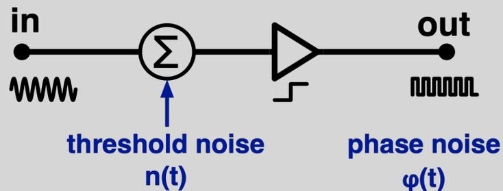
Sinusoid of peak amplitude  $V_0$  results in phase-type noise
