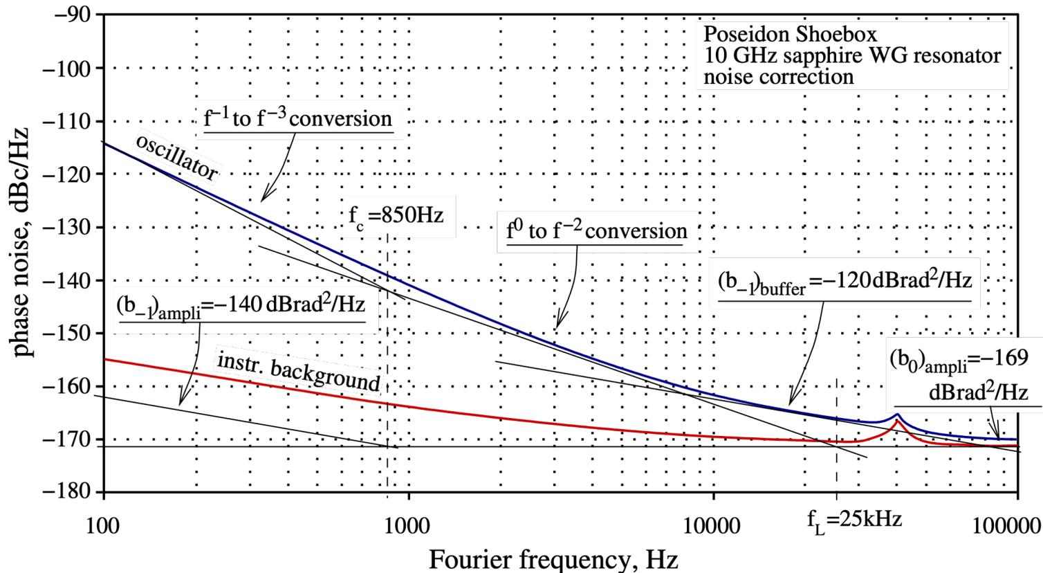
The  $1/f$  noise of the output buffer is higher than that of the sustaining amplifier (a complex amplifier with interferometric noise reduction / or a Pound control)
