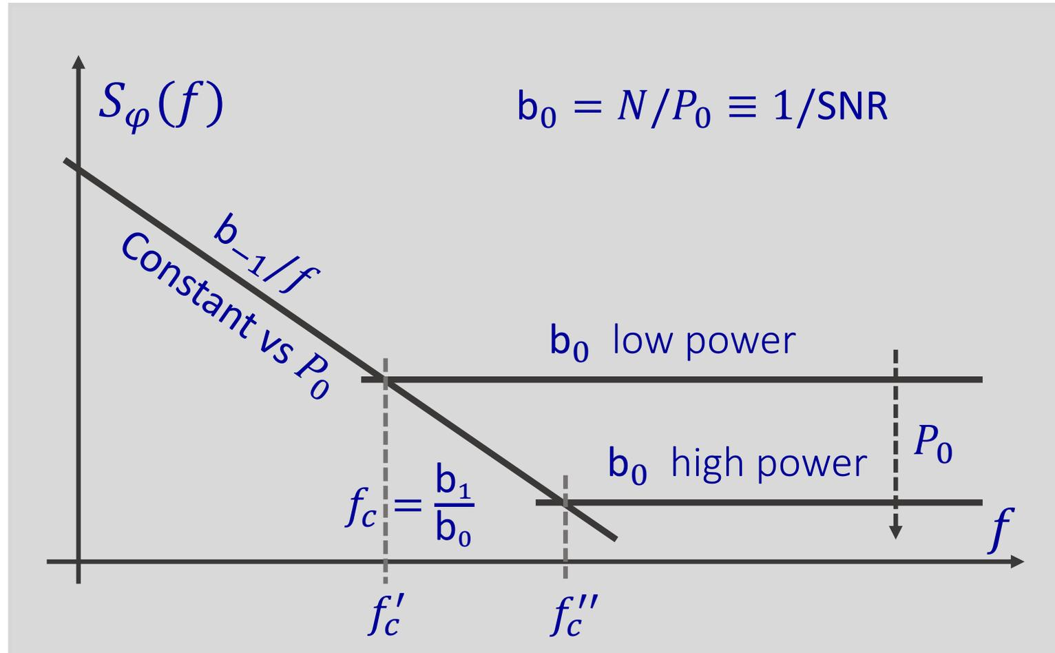
The corner frequency  $f_c$ , sometimes specified in data sheets is a misleading parameter because it depends on  $P_0$
