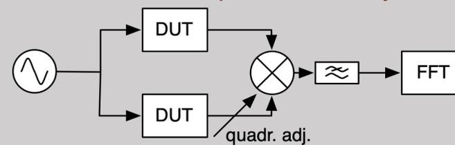
the measurement of an amplifier
