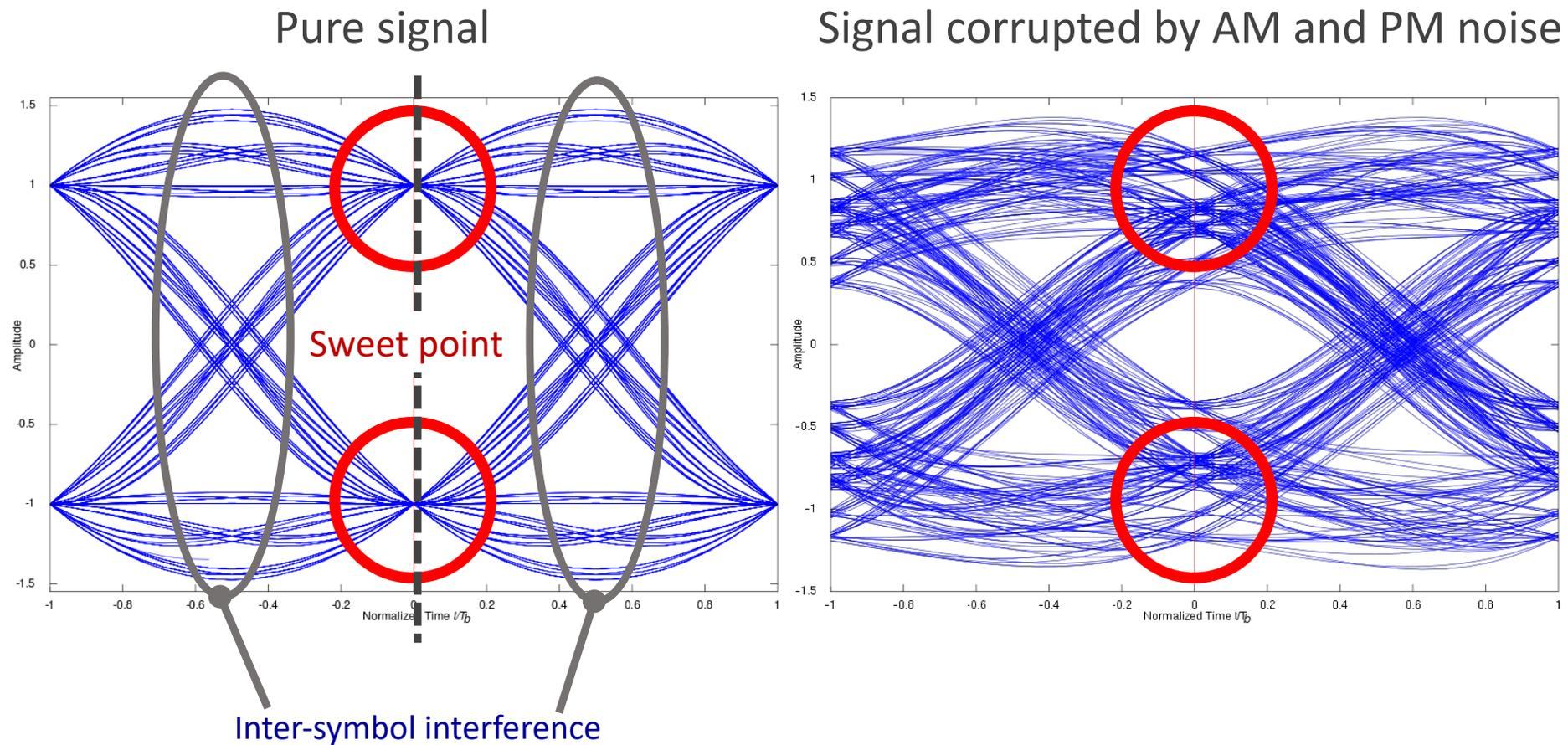
Timing impacts on the Bit Error Rate (BER)
