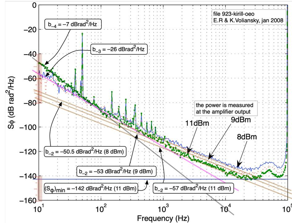
$$(S_\varphi)_{\min} = \frac{8}{m^2} \left\{ \frac{Fk_B T_0}{R_0} \left[ \frac{h\nu_l}{q\eta} \right]^2 \frac{1}{P_l^2} + 2 \frac{h\nu_l}{\eta} \frac{1}{P_l} \right\}$$
