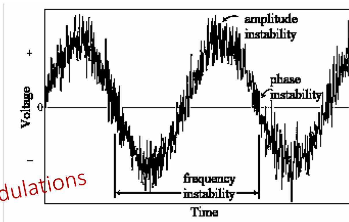
**Figure A.1—Instantaneous output voltage of an oscillator**
