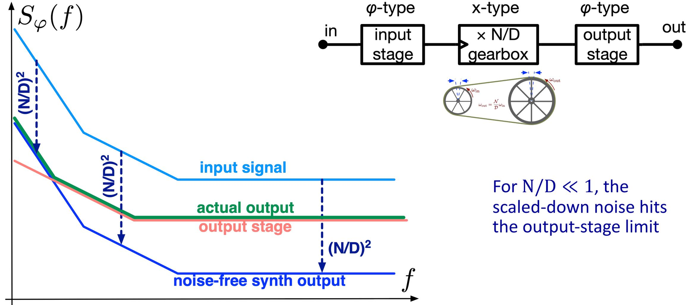
For  $N/D \ll 1$ , the scaled-down noise hits the output-stage limit
