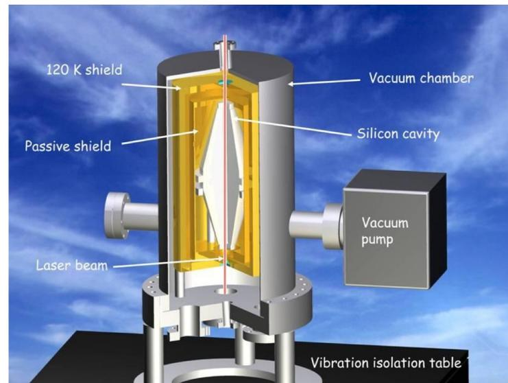
**Silicon cavity is thermally isolated by two gold-plated copper shields.**
