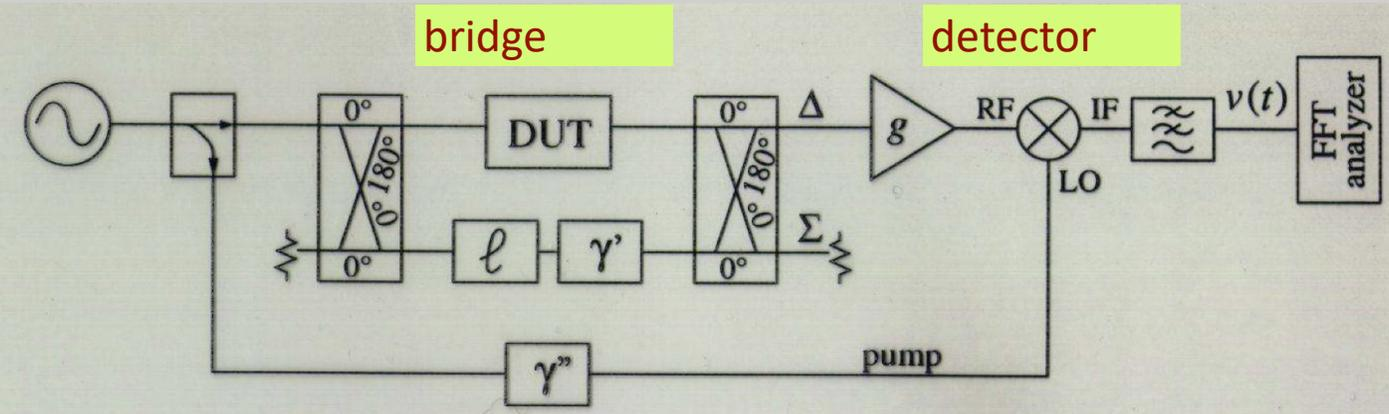
and rejection of the master-oscillator noise
