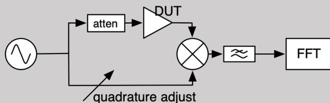
the measurement of a low-power DUT
