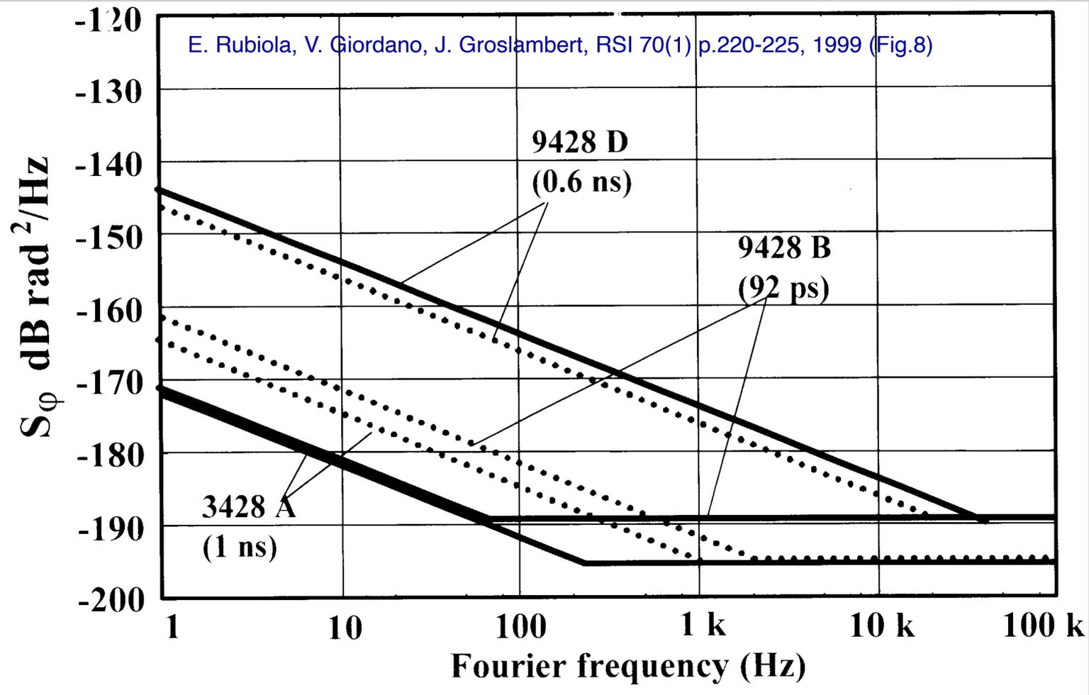
Microwave line stretchers measured at 100 MHz (all devices are manufactured by Arra)
