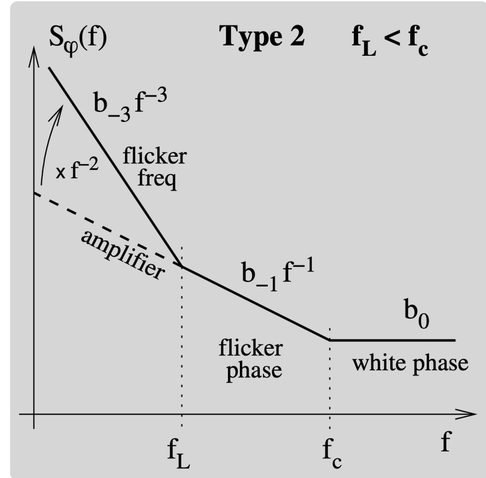
The sustaining-amplifier noise is  $S_\varphi(f) = b_0 + b_{-1}/f$  (white and flicker)
