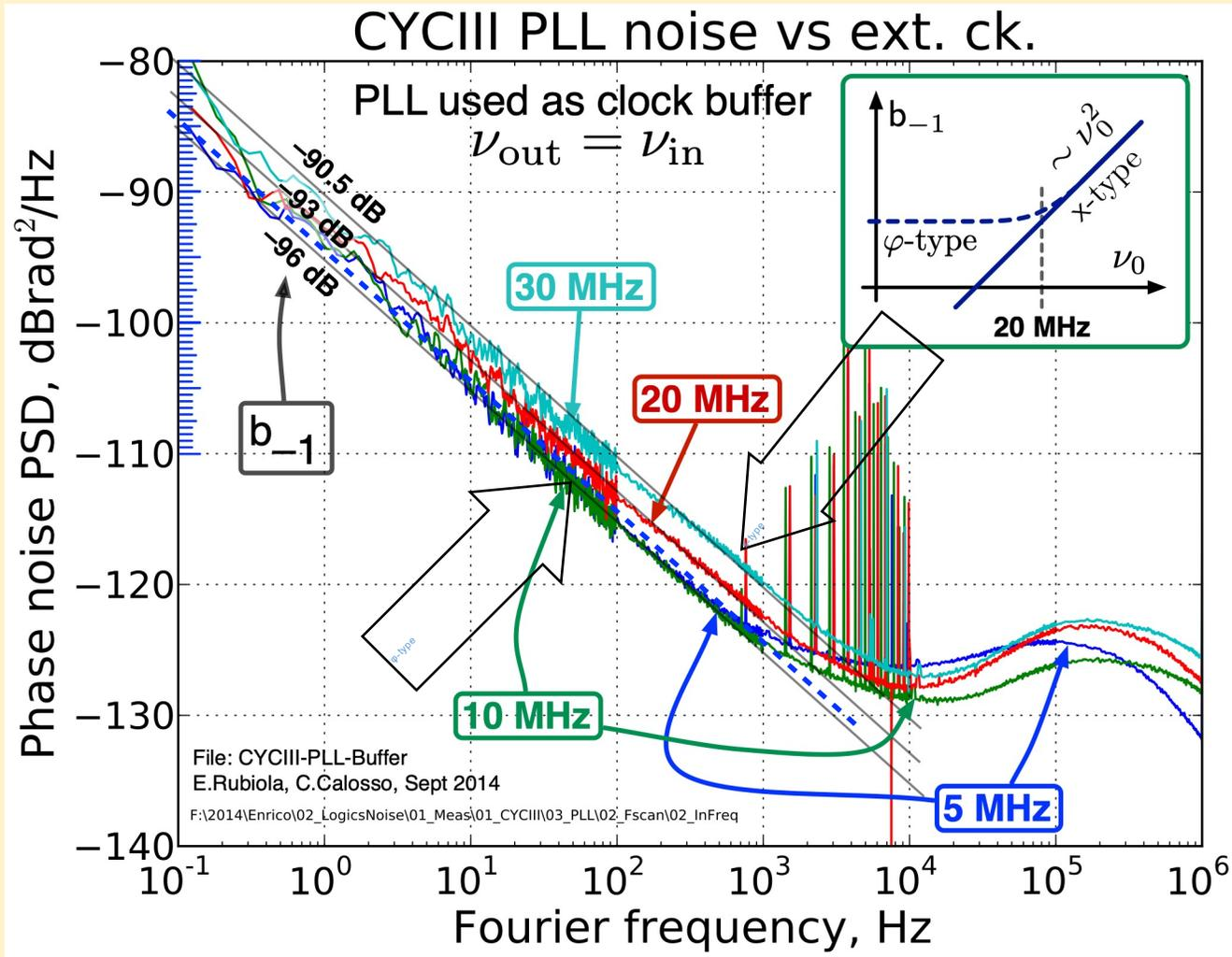
x-type → analog noise in the phase detector
