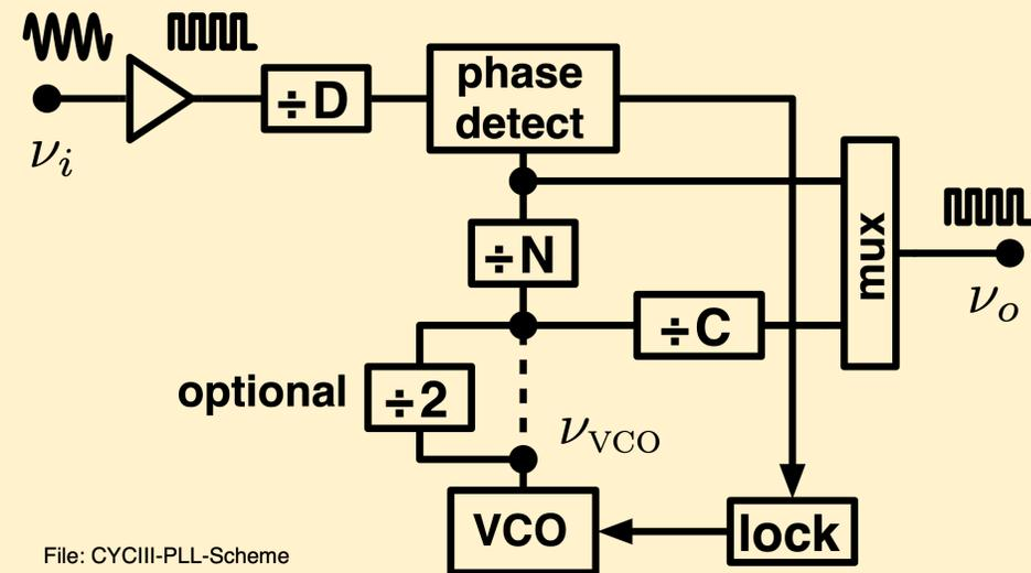
10 MHz input,  $N \times 10$  MHz out
