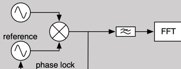
measure an oscillator vs. a resonator
