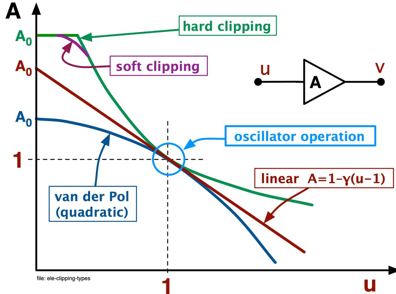
Gain compression is necessary for the oscillation amplitude to be stable
