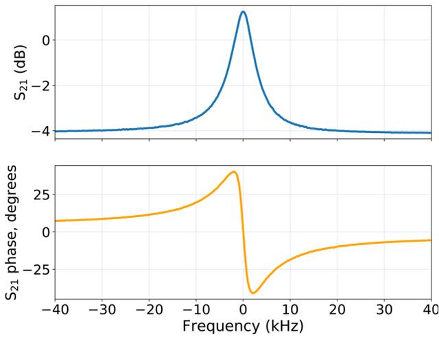
**FIG. 2.** Total gain and phase ( $S_{21}$  parameter, magnitude and phase) of the system, measured with a network analyzer in the open loop configuration (input: E, output: D). The center of the frequency axis corresponds to an atomic resonance frequency  $\nu_0 \sim 9.192\,640$  GHz, shifted from the exact Cs clock transition frequency due to the presence of buffer gas in the cell. A 100-pt averaging was applied onto the data.
