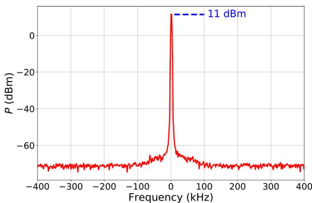
**FIG. 3.** Output spectrum of the CPT atomic feedback oscillator, measured at point B, for a laser power in the cell of 1.3 mW. The resonance occurs at the frequency of about 9.192 640 GHz. Parameters of the analyzer are: resolution bandwidth (RWB) = 3 kHz, video bandwidth (VBW) = 100 Hz, and sweep time = 0.2 s.
