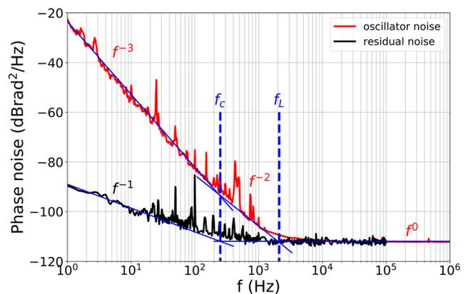
**FIG. 4.** Absolute phase noise at 9.192 GHz of the Cs cell atomic feedback oscillator (red line) and residual phase noise of the sustaining loop (black line). The measured Leeson frequency  $f_L$  is about 2.1 kHz, slightly lower than the calculated one  $f_L = \nu_0/2Q_L = 2.8$  kHz. The transition from the  $f^{-3}$  to the  $f^{-2}$  slope is obtained around the corner frequency  $f_c$  of the residual noise.
