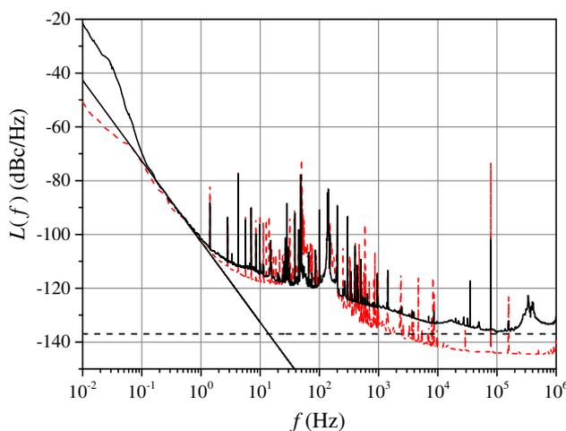
**Fig. 2.** Phase noise of the all-optical microwave signal compared to a CSO signal. *Black curve*: phase noise spectrum of the beat note between the CSO and the cavity signals. *Black line*:  $f^{-3}$  fit of the spectrum between 0.2 and 0.7 Hz. *Red dashed curve*: phase noise spectrum of the beat note between two identical CSOs. *Dashed line*: photodetection shot noise limit.
