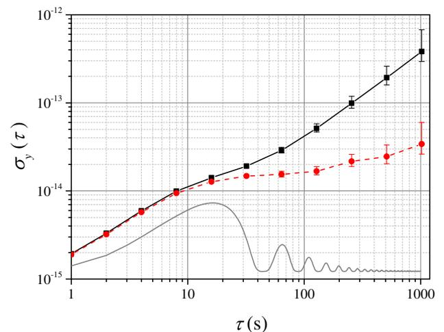
**Fig. 3.** Allan deviation of the all-optical microwave signal compared to a CSO signal. *Red dashed curve*: relative frequency stability with linear drift removed. *Light gray curve*: estimated contribution of the 26 mHz modulation to the Allan deviation.
