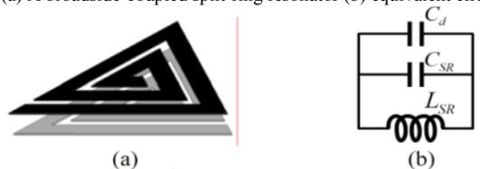
Fig.14: (a) Layout of the BCTSR (dark region denotes BCTSR etched on signal plane, and light region denotes broadsides coupled triangular SR etched on ground plane) (b) equivalent lumped circuit
