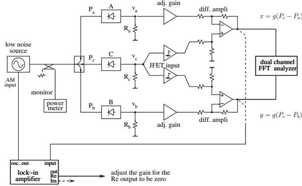
Fig. 3. Measurement scheme
