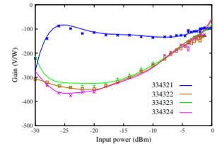
Fig. 6. Gain of 4 Schottky diode power detectors
