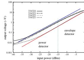
Fig. 5. Transfer functions of 4 Schottky diode power detectors
