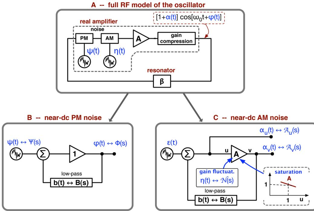
Fig. 1. Feedback oscillator and its decomposition in PM and AM models.
