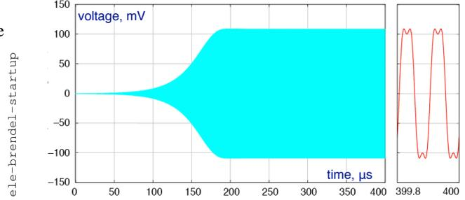
Fig. 11. Simulated oscillator startup.
