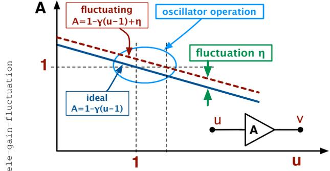
Fig. 8. Parametric fluctuation of the amplifier gain.
