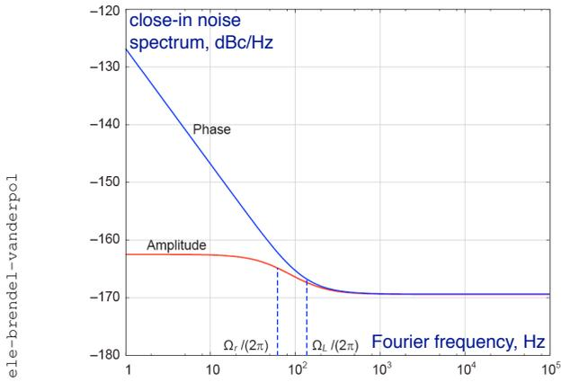
Fig. 12. Simulated van der Pol oscillator.
