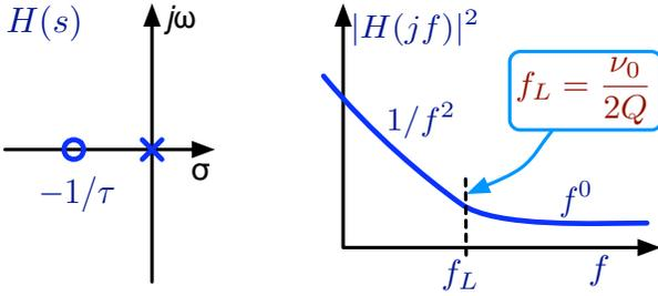
Fig. 4. Phase-noise transfer function.
