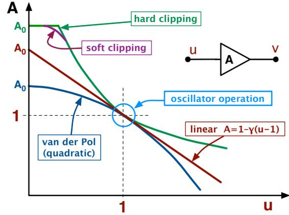
Fig. 6. Most common types of gain saturation. The quantities  $u$  and  $v$  are the rms amplitude at the carrier frequency.
