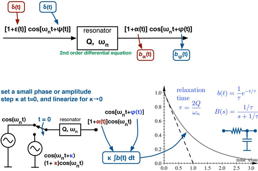
Fig. 2. AM and PM response of a resonator.
