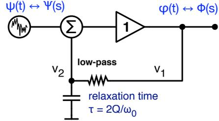
Fig. 3. Phase-noise model of the feedback oscillator.
