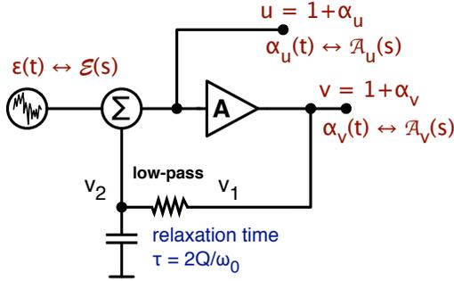
Fig. 5. Amplitude-noise model of the feedback oscillator.
