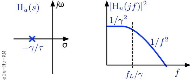
Fig. 9. Amplitude-noise transfer function (amplifier input).
