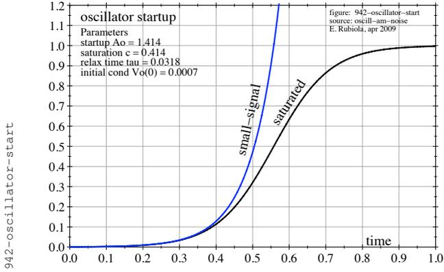
Fig. 7. Oscillator startup.
