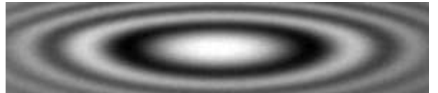
FIG. 4: Contour curves of the surface roughness resonator (fringe periodicity : 120 nm)
