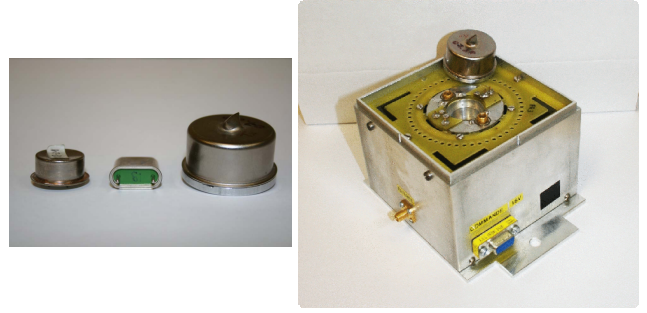
Figure 4. On left: various resonator cases (HC40, HC12, 5 MHz BVA). On right: the lower part of one resonator oven whose HC40 housing is visibly smaller than the 5 MHz BVA enclosure lied aside.
